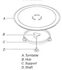
The turntable rotates in both directions to help cook food more evenly. Do not operate the microwave oven without having the turntable in place. See "Assistance or Service" to reorder any of the parts.
