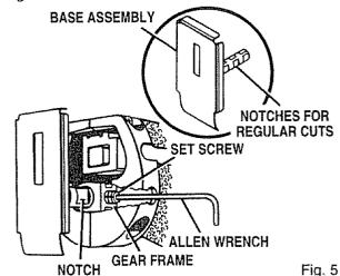
The base assembly of your electronic reciprocating saw is adjustable, allowing the use of the blade teeth at different positions on the blade.
