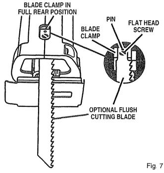
Tighten flat head screw securely.
