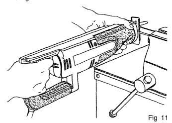
Metals such as sheet steel, pipe, steel rods, aluminum, brass, and copper may be cut with your saw. Be careful not to twist or bend the saw blade. **Do not force.** We recommend cutting oil when cutting most soft metals and steel. Cutting oil will also keep blades cool, increase cutting action, and prolong blade life.
