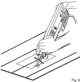
Mark the line of cut clearly. Choose a convenient starting point inside the area to be cut out and place the tip of the blade over that point. Rest front edge of base assembly on work and hold firmly in position.
