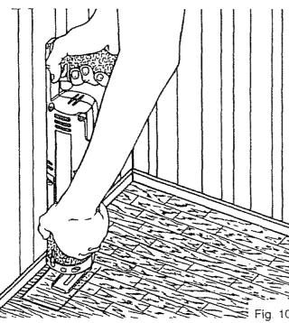
Your saw has been designed with a flush cutting feature which permits cutting close to floors or walls. To fit your cutting requirements, cuts may be made in either direction by reversing the position of the blade in the blade clamp. See page 10 for instructions on installing Flush Cutting Blade
