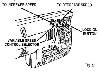
Your saw is equipped with a lock-on feature, which is convenient when continuous cutting for extended periods of time is required. To lock-on, depress the switch trigger, push in and hold the lock-on button located on the side of the handle, then release switch trigger. Release lock-on button and your saw will continue running.
