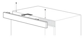
Remove the screw located above the door near the center of the oven that secures the bulb holder.
