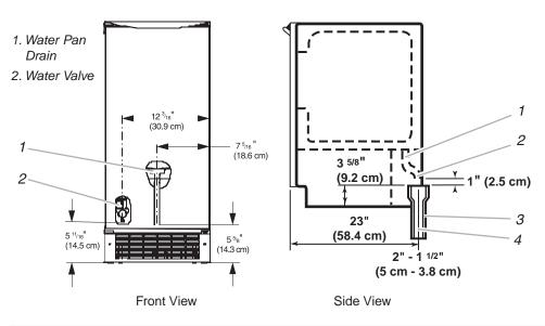
Drain lines must have a minimum of 5/8 in. (15.88 mm) inside diameter.
