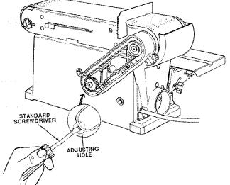
Test belt tension by placing fingers on either side of belt and squeeze. There should be about a 1/4" give to the belt.
