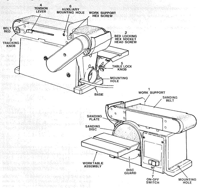
WARNING: To avoid injury from accidental start, turn switch "OFF" and remove plug from power source outlet before making any adjustments.
