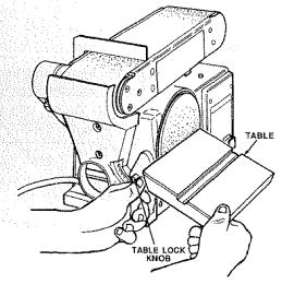
WARNING: To avoid trapping the work or fingers between the table and sanding surface, the table should be repositioned on the table support to retain a maximum of 1/16 inch distance between sanding surface and table.
