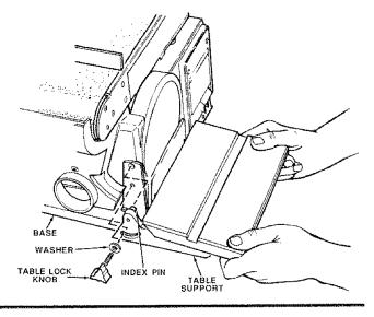
WARNING: To avoid trapping the work or fingers between the table and sanding surface, the table edge should be a maximum of 1/16 inch from sanding surface.
