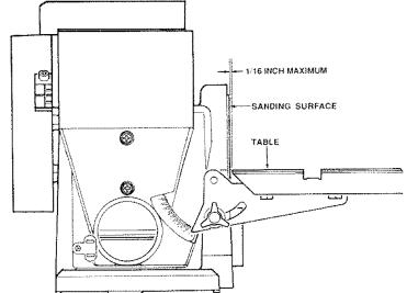
8. Use your Owner's Manual as a spacer. Place ten pages of the Owner's Manual between the Disc and the front edge of the table. Hold the table against the manual and tighten the three (3) Hex Washer Head screws.
