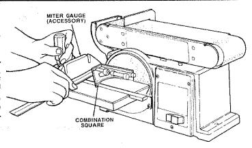
Always position the workpiece to the left of center on sanding disc with disc rotating counterclockwise as shown.
