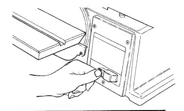
4.To lock switch in OFF position . . . hold switch IN with one hand . . . REMOVE key with other hand.
