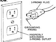
This power tool is equipped with a 3-conductor cord and grounding type plug listed by Underwriters' Laboratories. The ground conductor has a green jacket and is attached to the tool housing at one end and to the ground prong in the attachment plug at the other end. If repair or replacement of the electric cord or plug is necessary, do not connect the equipment grounding conductor to a live terminal.
