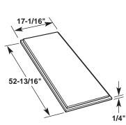
Cut door panel as shown. If the desired panel is greater than 1/4" thick, rout a 1/4" thick edge, in 1/4" from all four edges.
