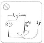
Do not damage electrical cable itself or place heavy objects on the cable.
