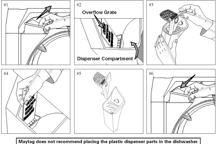
laytag does not recommend placing the plastic dispenser parts in the dishwasher. If laundry additives were on the parts when washed in the dishwasher, they may cause oversudsing in the dishwasher.
