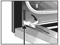
Lock engaged for door removal Figure 2
