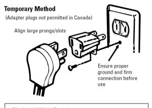
**CAUTION:** Attaching the adapter ground terminal to the wall receptacle cover screw does not ground the appliance unless the cover screw is metal, and not insulated, and the wall receptacle is grounded through the house wiring. The customer should have the circuit checked by a qualified electrician to make sure the receptacle is properly grounded.
