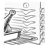
The oven has a special low shelf (R) position just above the oven bottom. Use it when extra cooking space is needed, for example, when cooking a large turkey. The shelf is not designed to slide out at this position.
