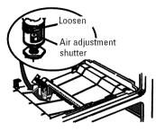
The shutter for the bottom (oven) burner is near the back wall behind the warming drawer. Remove the drawer. See the *Care and cleaning of the range* section.
