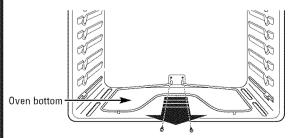
**D.** Lift the rear of the oven bottom enough to clear the lip of the range frame, push it back, and then pull it up and out.
