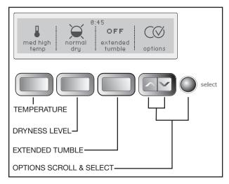
Auto Dry cycles take the guesswork out of selecting the correct drying time for each load. Moisture sensing bars at the back of the dryer drum sense the moisture level of the load as it tumbles through the heated air. With Auto Dry cycles, the load will automatically be dried at the selected temperature to the desired dryness level.
