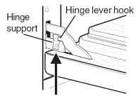
Lock engaged for door removal Figure 1
