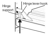
Lock engaged for door removal Figure 1
