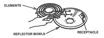
CAUTION: Do not pull element up more than 1/2" or damage to the receptacle will occur.
