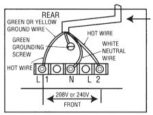
POWER SUPPLY CORD 4 #10 AWG MINIMUM COPPER CONDUCTORS, 30 AMP, 240V, WITH CLOSED-LOOP TERMINALS TYPE UL RECOGNIZED MINIMUM RATED 90°C.
