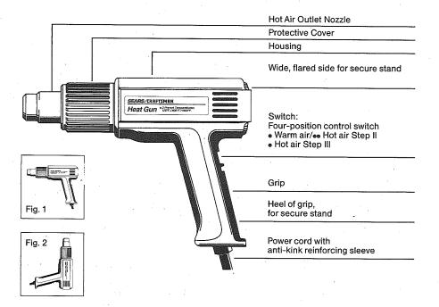
To operate the Heat Gun, plug the cord into a 120 Volt, 60 Hz, AC, power source. Be sure the power switch is in the OFF position.
