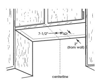
**To wire through top,** mark a line 7-1/2" from the right of the centerline on the underside of the cabinet. Mark the point on this line that is 2" from back wall. Drill a 1-1/4" diameter hole through the cabinet at this point. Note: If a cord-connection kit is used, drill a 1-5/8" diameter hole.
