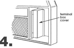
If your model does NOT have a factory installed power cord, remove terminal box cover from range hood.
