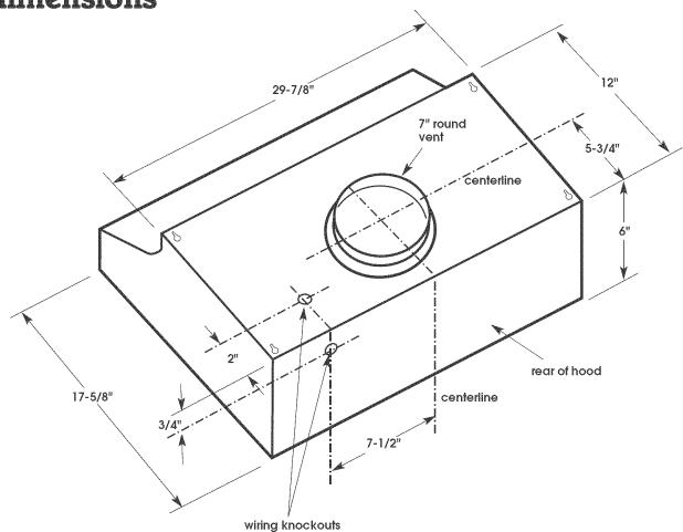
A 115-volt, 60-Hz, AC-only, fused electrical supply is required. The total ampere load used, including the range hood, must not exceed 90% of the rated capacity of the circuit. The ampere rating of the range hood is located on the model/serial number rating plate located on the side cover of the fan motor housing.
