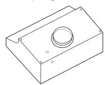
If roof or wall cap does not ■ have a damper, install damper (supplied with hood) in vent system to prevent air from flowing back into vent
