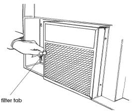
Pull firmly on filter tab to remove filter/light lens from range hood..
