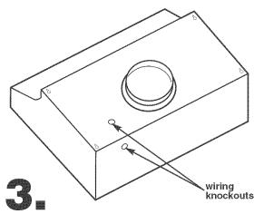
Remove knockout from the wiring opening (top or rear) to be used.
