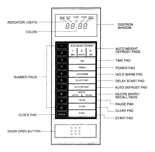
**NOTE:** To enter a setting, touch a word or number pad. A beep sounds when a pad on the control panel is touched to indicate a setting has been entered.
