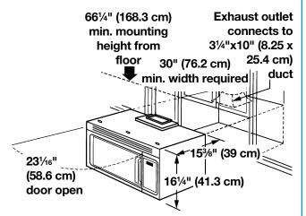
Shipped ready for ventless (recirculating) operation, converts to top or rear discharge.
