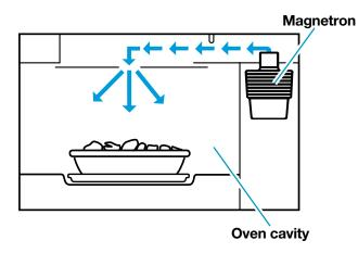
The glass turntable of your microwave oven lets microwaves pass through. Then they bounce off a metal floor, back through the glass turntable, and are absorbed by the food.
