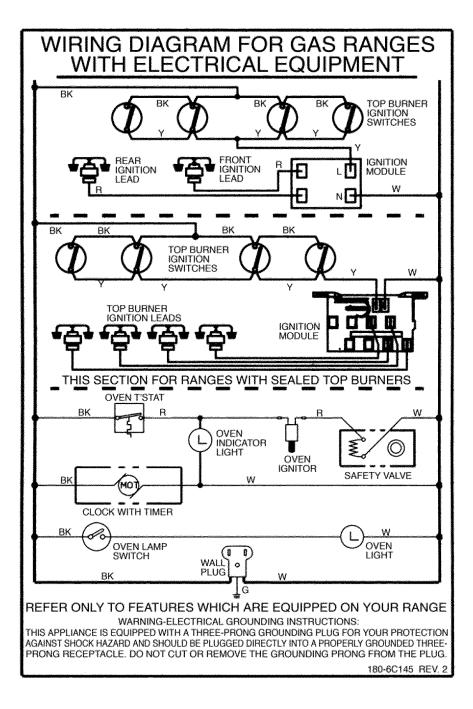
Refer to this diagram for ranges equipped with top burner spark ignition and glow coil oven ignition.
