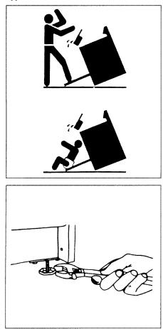
**AWARNING** To reduce the risk of tipping the appliance by abnormal usage or improper door loading, the appliance must be secured by properly installing the anti-tip device packed with the appliance. To check if the device is installed and engaged properly, carefully tip the range forward. The Anti-Tip device should engage and prevent the range from tipping over.
