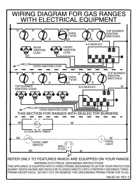
Refer to this diagram for ranges equipped with all spark ignition.
