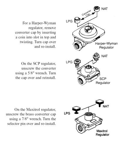
**Note:** What you read on the converter cap or plunger is the type of gas for which the regulator is set. If yours reads NAT, the regulator is set for natural gas. If yours reads LP, the regulator is set for LP.
