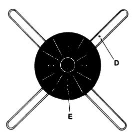
The removable filter continuously filters the wash water and traps the food particles that have been removed from the dishes on the outside of the filter. These trapped food particles are removed from the filter by the jet spray action of water from the single spray nozzle (D) underneath the wash arm. The ultrafine filter is cleaned by the nine water jets (E) underneath the 4-Way Hydro Sweep Wash Arm.
