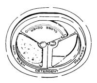
Fill the Main Wash compartment for the Light / China Wash Cycle when the dinnerware is lightly soiled.
