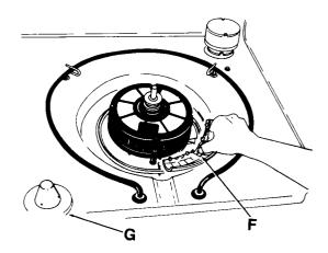
The coarse strainer may be removed, if necessary. To remove, lift strainer out by squeezing center section (F) and remove. To replace, squeeze center section so clips snap into square notch.
