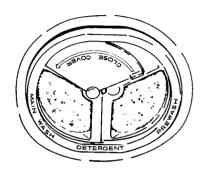
Add detergent to both the Prewash and Main Wash compartments for the Light / China Wash Cycle, the Normal Wash Cycle and the Pots / Pans Cycle when dishes are heavily soiled.
