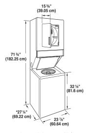
\*Most installations require a minimum 5½" (14 cm) clearance behind the dryer for the exhaust vent with elbow. See "Venting Requirements."
