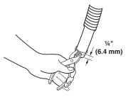
**4.** Open clamp. Twist hose back and forth while pushing onto drain connector on the side of the washer/dryer. Continue until hose contacts the ribbed stops on the cabinet.
