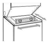
If the washer/dryer is not level, prop up the front with a wood block and adjust the feet up or down as necessary. Remove wood block and lower washer/dryer. Repeat this step until the washer/dryer is level.
