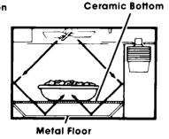
The ceramic bottom of your microwave oven lets microwaves through. Then they bounce off a metal floor, back through the ceramic bottom and are absorbed by the food.
