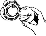
4. Replace the bulb cover and snap the wire holder into place. Plug in appliance or reconnect at the main power supply.
