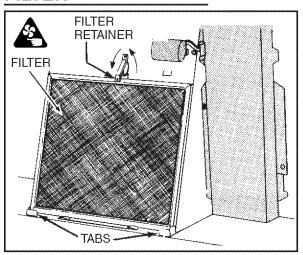
Remove aluminum filter by turning filter retainer to one side. Filter should be washed once a month in a hot detergent solution. Aluminum filters are dishwasher safe. When installing filter, make sure that filter slides under retaining tabs on back of fan housing. Turn filter retainer so that arrows on retainer point toward front and back of hood.
