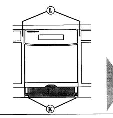
near the console (**J**). Tilt dishwasher backwards on wheels. Move dishwasher close to cabinet opening. Do Not push on the center of the console. Discard shipping base or hardboard.
