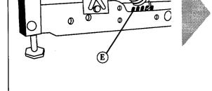
easily. If door closes too quickly or falls open, adjust door springs (D) by moving spring ends to different holes (E) in base.
