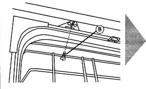
The dishwasher MUST be secured to countertop or floor to keep it from tipping when door is opened.
