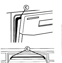
Open door about 3 inches (7.6cm) and check for equal spacing (C) between inner door and tub sides. If spacing is not equal, loosen bracket screws and shift tub. Tighten bracket screws. Remove newspaper or towel from dishwasher.
