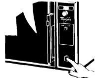
5. Push the START Button. The oven light will come on. You will hear a fan running during oven operation.
