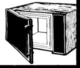
**DO NOT** operate the oven if it is damaged. It is particularly important that the oven door close properly and that there is no damage to the (1) Door (bent),
