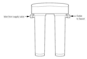
3 Push the tubing firmly into each fitting on the manifold until the line is flush with the fitting collar. (If the tubing is removed, re-cut the end, measure, mark and re-insert). Tubing must be fully inserted to avoid leaks (Fig. 11). (To remove tubing, depress and hold white collet, pull tubing out to remove.)
