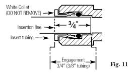
4 Pull out slightly on tubing to ensure a good seal.
