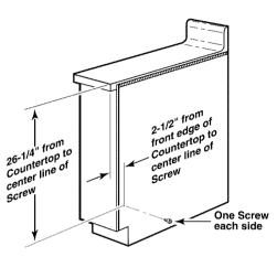
Carefully mark the cabinet for the location of the stop screws. Drill 1/8" pilot holes into the cabinet, each side of the range. (Make sure not to drill entirely through the cabinet wall.) Carefully turn the shoulder screws into the pilot holes until they are tight.
