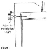
• Measure installation height and dishwasher height Extend leveling legs out from the dishwasher base, 1/2" less than installation height
