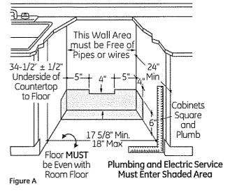
• The rough cabinet opening must be at least 24" deep. 17-5/8" to 18" wide and approximately 34-1/2" high from floor to underside of the countertop.
