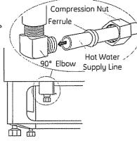
**IMPORTANT** – Check to be sure that door spring does not rub or contact the fill hose or water supply line. Test by opening and closing the door Re-route the lines if a rubbing noise or interference occurs
