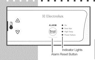
The electronic control system continuously monitors your refrigerator/freezer for temperature consistency, doors left ajar, and power failures. Variances from normal operating conditions are communicated by audible tones and a set of four status indicator lights.
