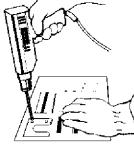
cm) drill bit to drill the two holes. Remove template from floor.
