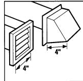
3. The exhaust vent can be routed up, down, left, right, or straight out the
