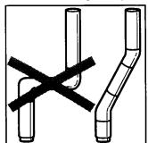
exhaust vent. Avoid 90° turns, if possible. Allow room when using elbows or making turns. Bend vent gradually to avoid kinking.
