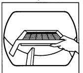
wall of the dryer. Lower the front so the legs rest on the dryer opening.
