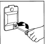
from the back wall of the dryer by removing the screw located in the lower right corner of the cover.
