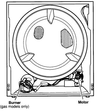
Dryer with front panel removed
