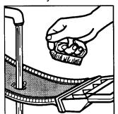
detergent; scrub lint screen with the brush to remove residue buildup.
