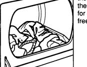
the door. Do not pack the dryer; allow space for clothes to tumble freely.
