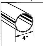
be used. **Do not** use plastic vent or flexible metal foil vent. Do not kink or crush flexible metal vent. It must be completely extended to allow adequate exhaust air to flow. Check vent after installation. Refer to your Installation Instructions for proper
