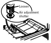
The shutter for the bottom (oven) burner is near the back wall behind the warming drawer, storage drawer or kick panel. Remove the drawer or panel. See the *Care and cleaning of the range* section.
