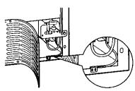
**IMPORTANT:** To ensure a proper ground, the end of the ground wire **MUST** be secured to the refrigerator cabinet.
