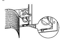
**IMPORTANT:** To ensure a proper ground, the end of the ground wire **MUST** be secured to the refrigerator cabinet.
