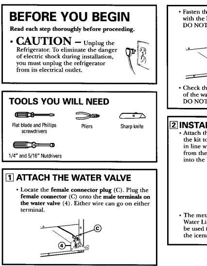
• Fasten the water valve to the cabinet edge hole with the **hex-head screw** (13) from the kit. DO NOT DRILL ANY ADDITIONAL HOLES.
