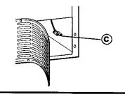
• Plug the **female connector** (C) onto the **male terminals on the water valve** (3). Either wire can go on either terminal.
