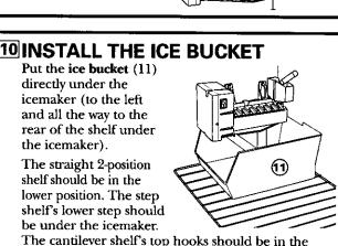
The cantilever shelf's top hooks should be in the 6th slot up from the bottom of the track.
