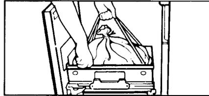
4. Remove bag carrier handles from side retainers and hold. **For easy bag removal**, release side of drawer by opening the latch at the right front. Lift bag and carrier out of drawer.
