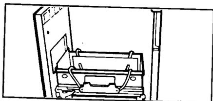
2. Fit the bag carrier in the drawer. Tuck the rope handles behind the bag retainers as shown.
