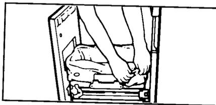
5. Lock bag in place by tucking cuffs behind bag retainer and by pulling the four prepunched holes over the bag retainer buttons. Holes will expand over the buttons without harming the bag.
