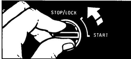
**Before cleaning the compactor,** turn the key-knob to the STOP/LOCK position and remove.
