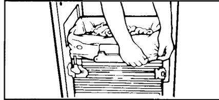
2. Remove top of bag from bag retainers and bag retainer buttons. Pull up all four bag cuffs.
