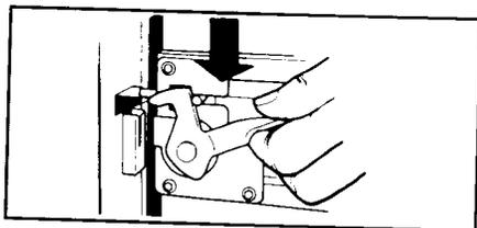
1. Push side of drawer closed, then latch the drawer side by pushing the latch up.
