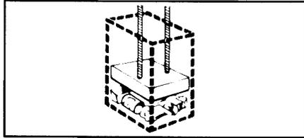
The compacting ram does not go to the drawer bottom. You will not see compacting of the first few loadings.
