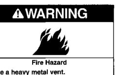
Do not use a plastic vent. Do not use a metal foil vent. Failure to follow these instructions can result in death or fire.
