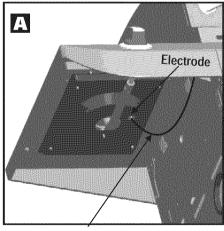
Sideburner Ignitor Wire
