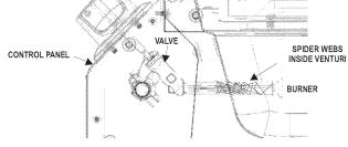
In some areas of the country, spiders or small insects have been known to create "flashback" problems. The spiders spin webs, build nests and lay eggs in the grill's venturi tube(s) obstructing the flow of gas to the burner. The backed-up gas can ignite in the venturi behind the control panel. This is known as a flashback and it can damage your grill and even cause injury.
