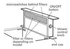
16. Push and hold for a few seconds the button on the top of the downdraft vent. Retractable section of downdraft vent will rise and blower will start. Position the top trim over the retractable section and snap trim into place.
