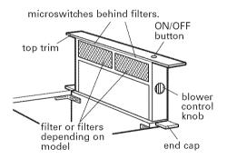
15. Push and hold for a few seconds the button on the top of the downdraft vent. Retractable section of downdraft vent will rise and blower will start. Position the top trim over the retractable section and snap trim into place.
