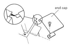
**3.** Attach the left side and right side end caps to the downdraft. Use 1 screw with each end cap.
