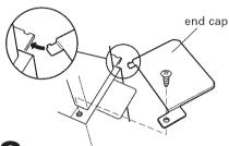
3. Attach the left side and right side end caps to the downdraft. Use 1 screw with each end cap.
