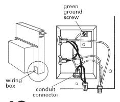
Remove required knockout and install conduit connector. Feed the power supply cable through the conduit connector and into the wiring box. Connect the white wires together with a twist-on wire connector. Connect the black wires together with a twist-on wire connector. Attach the green (or green and yellow) ground wire to eyelet with green ground screw. Tighten the conduit connector clamp screws. Replace the wiring box cover.
