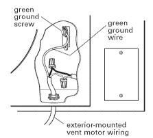
**14.** Remove vent box knockout and install conduit connector.
