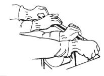
Carefully insert downdraft vent into countertop cutout. Two people are recommended to support the weight of the downdraft vent during lifting. Check that downdraft vent is parallel to side of cutout and that mounting brackets rest gently on countertop.
