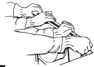
Carefully insert downdraft vent into countertop cutout. Two people are recommended to support the weight of the downdraft vent during lifting. Check that downdraft vent is parallel to side of cutout and that mounting brackets overlap countertop.
