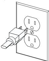
**OUTLET RECEPTACLE** - Properly grounded 3-prong receptacle to be located so the power supply cord is accessible when the washer is in an installed position. NOTE: GFI (Ground Fault Interrupter) receptacle is not required.
