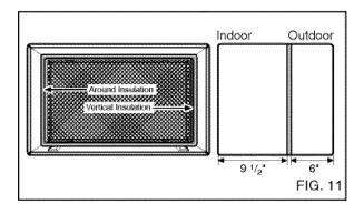
If the depth of your existing wall sleeve is less than or equal to 18", skip to step 6. Otherwise, cut the baffles and the support blocks according to length "A" in the table below.
