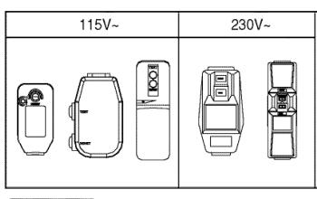
Power cord may include a current interrupter device. A test and reset button is provided on the plug case. The device should be tested on a periodic basis by first pressing the TEST button and then the RESET button. If the TEST button does not trip or if the RESET button will not stay engaged, discontinue use of the air conditioner and contact a qualified service technician.
