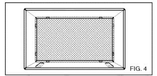
Fasten the 4 washer screws to secure the grille to the wall sleeve. If you need plastic nuts to mount plastic grille to the inside of the wall sleeve, there are plastic nuts in the installation kit. The nuts are installed from the inside of the sleeve and are pressing into the square holes of the rear flanges.
