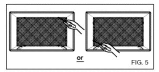
Remove the backing from the Vertical Insulation strip  $159/16 \times 13/8 \times 13/8$  and attach that to the inside right of the sleeve as shown below. Remove the backing from the Around Insulation strip  $67^{1}/_{8}$  x  $1^{3}/_{8}$  x  $^{25}/_{32}$  and attach that to the inside front of the sleeve as shown below.
