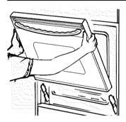
The oven door is removable for easier access to the light bulb. Lift the door straight up and off the hinges.
