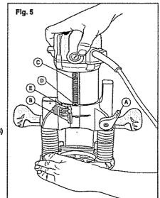
NOTE: When making depth adjustments on the plunge base, the motor clamp should always be closed securely.
