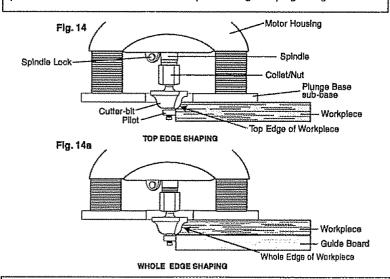
⚠ WARNING: Always securely clamp your workplece and keep a firm grip on the router base with BOTH HANDS at all times. Failure to do so could result in loss of control causing possible serious personal injury.
