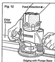
⚠ WARNING: Always securely clamp your workpiece and keep a firm grip on the router base with BOTH HANDS at all times. Failure to do so could result in loss of control causing possible serious personal injury.
