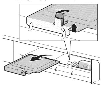
6. Remove old light bulb and replace only with equivalent 30 watt bulb available from parts distributor. Bulbs are also available at most hardware stores or lighting centers.
