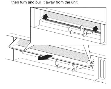
4. Remove the charcoal filter by pushing it inwards,
