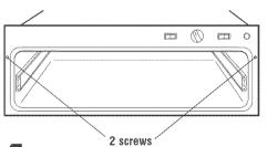
Use two (2) screws provided to secure the warming oven frame to the cabinet.
