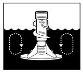
rollover action that provides a thorough cleaning of the wash load. After agitation starts, the Cycle Control knob turns clockwise until it points to an Off area and the cycle ends.
