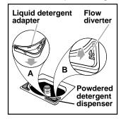
diverter (labeled A in illustration) and flow diverter (labeled B in illustration) into the powdered detergent dispenser. The dispenser holds 125 mL (1/2 cup).
