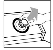
**NOTE:** To **stop** the washer at any time, push in the Cycle Control knob. Do not stop the washer during water pump out. To **restart** the washer, close the lid (if open) and pull out the Cycle Control knob.
