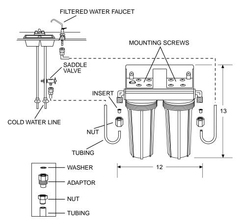
**Note:** Can be installed undercounter (as shown), in basement, or other convenient location. See installation instructions packed with product for complete details.
