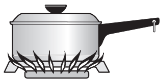
IMPROPER FLAME SIZE
