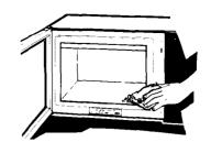
Be sure to clean the areas where the door and oven frame touch when closed. Rinse well.
