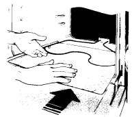
Slide the foil under the bake element.
