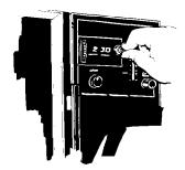
3. Set cooking times up to 10 minutes by **pushing in** the timer knob and turning clockwise. The oven light will go on. Push in and turn counterclockwise to reduce time.
