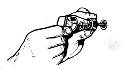
First make sure lower oven and surface unit control knobs are set on OFF. All knobs pull straight off. Surface unit knobs have a collar and spring.
