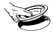
Hold the surface unit as level as possible with the terminal just started into the receptacle.
