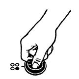
Line up openings in the reflector bowl with the surface unit receptacle and the element holddown clip.
