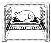
Use the convection roasting rack on the broiler pan and grid (all included with your oven). (The convection roasting rack rests on the broiler pan and grid.) The long side of the rack should be parallel with the oven door for best heat distribution and airflow.
